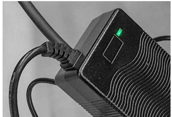
Charge the battery for 24 hours non-stop before using the trolley for the first time.
