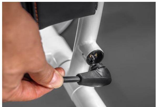
Connect the battery using the magnetic connector. The connector faces forwards horizontally. The flashing signal on the upper control unit indicates that the battery has been connected properly.
