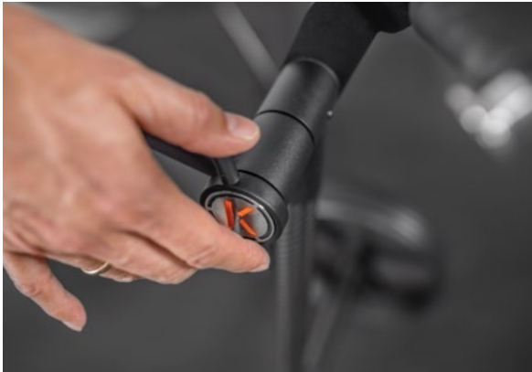
Securing the upper handlebar section
