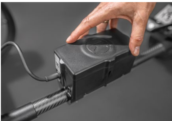
Front edge flush with the permanently mounted battery support.
